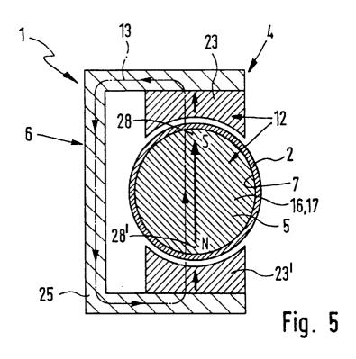
The invention relates to a drive device, comprising a tubular housing, on which a longitudinally moving movable unit is mounted, such unit having an inner part located in the interior of the housing and an outer part which is arranged externally on the housing and is magnetically coupled for movement with the inner part by means of a coupling means having at least one permanent magnet means.
