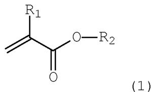
**[092]** wherin  $R_1$  is chosen from H or  $CH_3$  and  $R_2$  is H or an aliphatic or aromatic radical having at least one atom that is not C or H.
