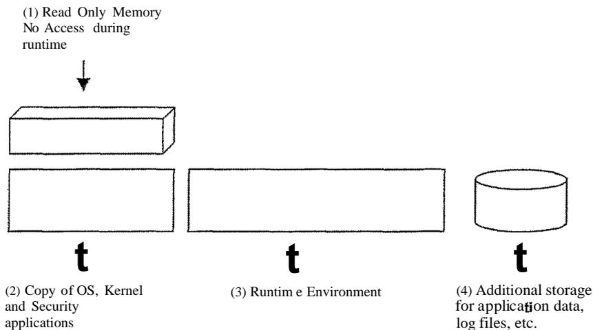
Upon each "hard" restart, the boot loader {resident at area 1} of the mobile security system 345 copies the kernel and security applications (a fresh unchanged copy) from area 1 to 2. This causes a clean version of the OS and applications to be loaded into area 2 each time. That way, if a special mobile security system 345 attack is developed, the attack will be unable to infect the
