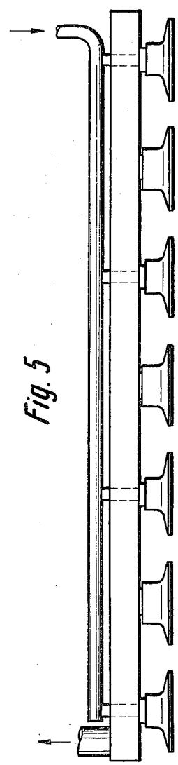
DEVICE FOR RAISING THE TOP SHEET OF A PILE
