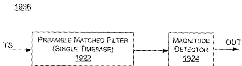
TIME BASE AND TIMING ACQUISITION COMPONENT FOR RECOVERING TAG'S PREAMBLE
