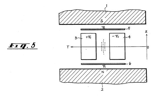
MASS SPECTROMETER WITH SUPERIMPOSED ELECTRIC AND MAGNETIC FIELDS
