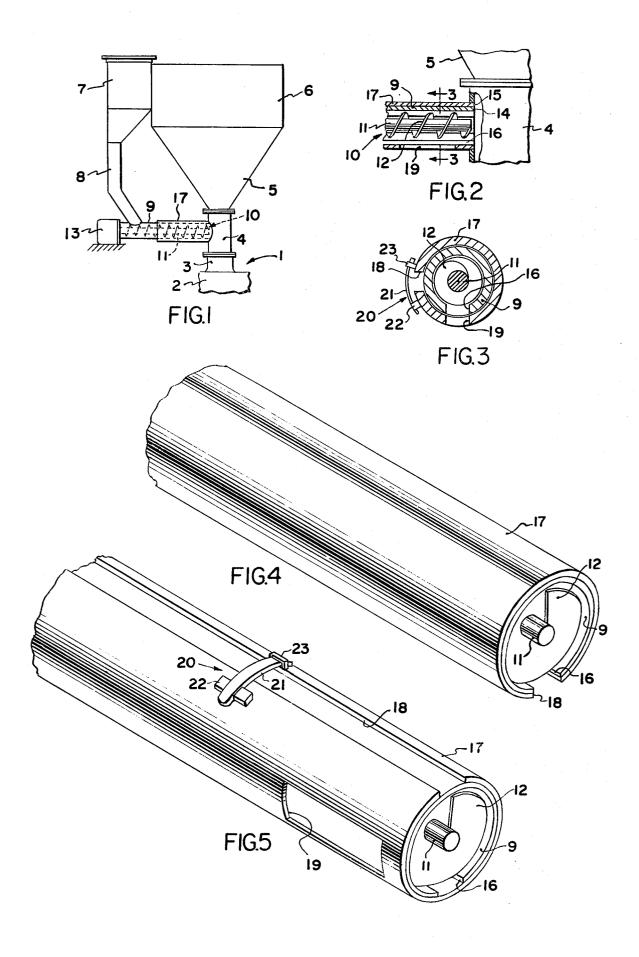
Shortening of the effective length of the tubular conduit is achieved by rotating the sleeve to a position in which the smaller opening is aligned with the conduit's slot and at a point between the ends of the conduit.
