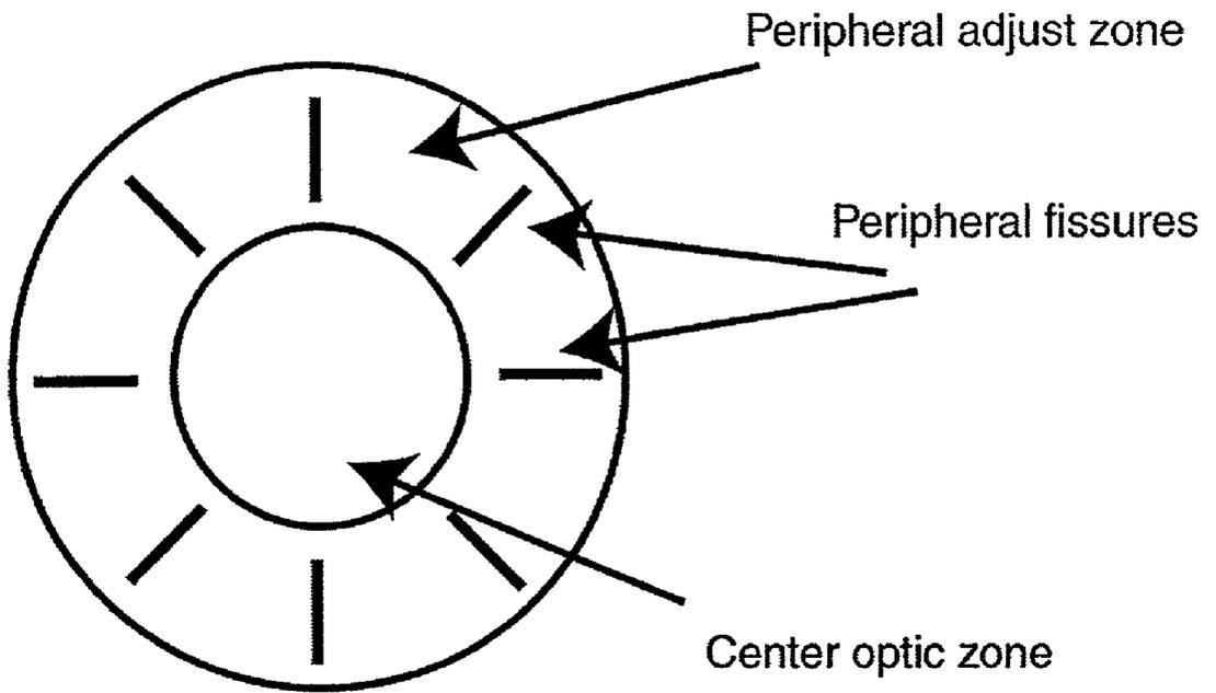
**Figure 3 Basic structure of adjustable optic surface**
