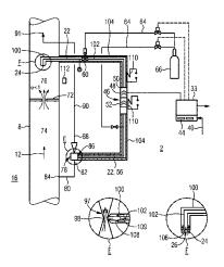
from there to the jet pump and connected to the pump fluid connector. A sample return line is guided from the functional path to the jet pump and connected to the suction connector.
