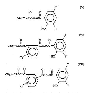
where R, Y, L and M are defined as above. The aforementioned monomers can be reacted as starting materials or, as explained below, they can be formed in situ by ligand exchange between an acidic monomer (e.g., acrylic or methacrylic acid) and a zinc salt (e.g., zinc salicylate, zinc 3,5 di-t-butyl salicylate, and the like) during polymerization of the acidic monomer.
