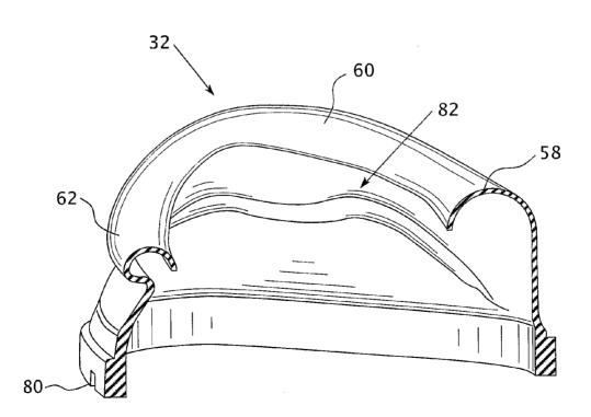
(57) **Abstract:** A respiratory mask (30) is provided having an outer shell (34) coupled to a cushion (32) for the delivery of a gas to a user. The cushion (32) of the respiratory mask (30) has a pleat (82) and varied wall thicknesses about the device in order to provide varying degrees of flexibility and support about the cushion (32).
