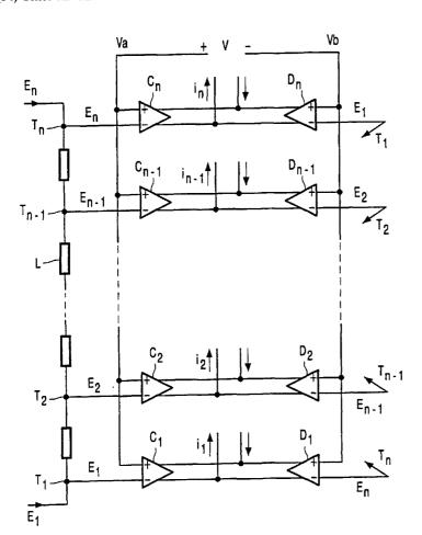
(57) Abstract: An analog to digital converter has a differential input arrangement with a static reference ladder and comparators for comparing the differential input signal with respective reference voltages from the ladder. For sensing the positive and the negative values of the input signal the same taps of the reference ladder are used.
