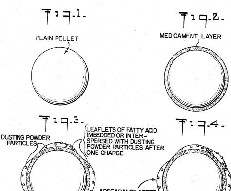
APPEARANCE AFTER 2 CHARGES NOTE OVERLAPPING LAYERS OF ACID WITH INTER-SPERSED DUSTING POWDER
