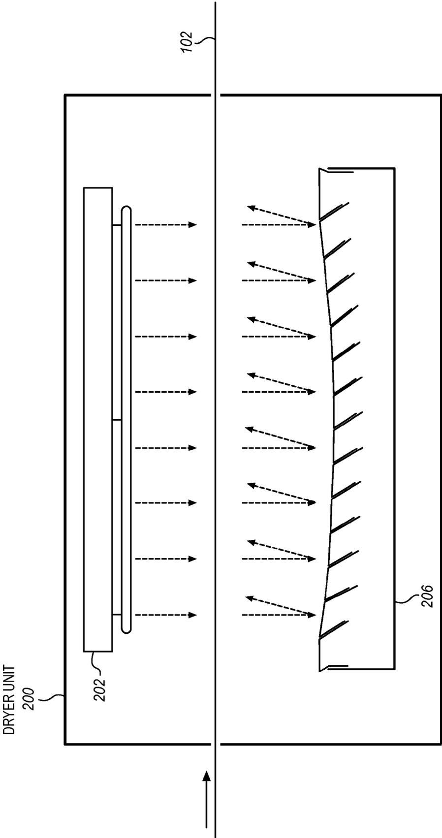
**REFLECTOR STRUCTURE FOR A RADIANT DRYER UNIT OF AN INKJET PRINTER**
