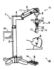
and returning from the eye and the reference light having passed through the reference optical path. The image forming unit forms an image of the eye based on a detection result obtained by the interference optical system.
