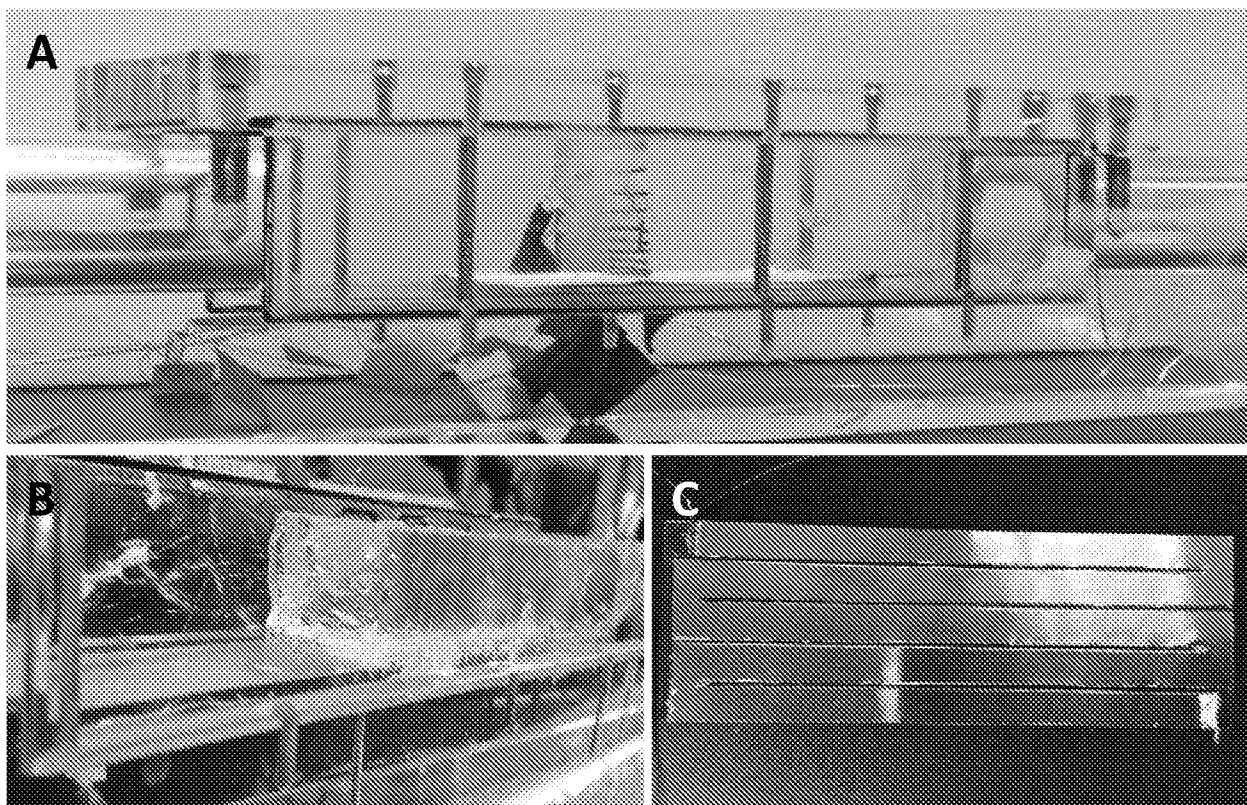
Acrylic chamber used for thermal model (A) 6.45 cm 2 cross-section of PVA hydrogel tissue mimic (B) 19.3 cm 2 -area, 25 μm-thick, nichrome foil heating element (C).
