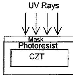
Step2 Mask is placed in contact with Photoresist
