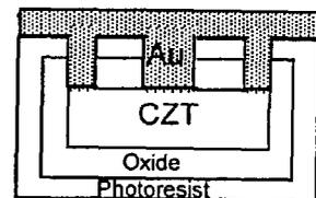
Step6 Gold is deposited on substrate
