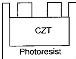
Step3 Photoresist is developed
