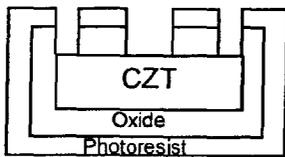
Step5 Oxide is etched through pattern photoresist
