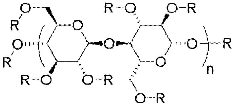
wherein each R is independently H or CH<sub>3</sub> and n is an integer having a value from about 34 to about 43 and wherein methoxy substitution is from 27.5% to 31.5% by weight.
