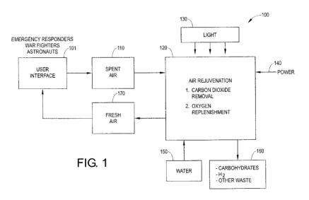
(57) Abstract: The present invention provides for carbon dioxide removal and fixation using a cell incorporating a carbon dioxide selective film for active/passive transport while simultaneously producing oxygen and an air bladder for use in battlefield applications and the like where oxygen requirements are often extreme.
