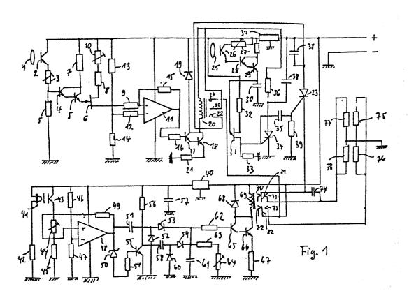
The invention concerns an apparatus for controlling the light of the headlights of a vehicle by controlling the current or voltage of the lamps of the headlights
