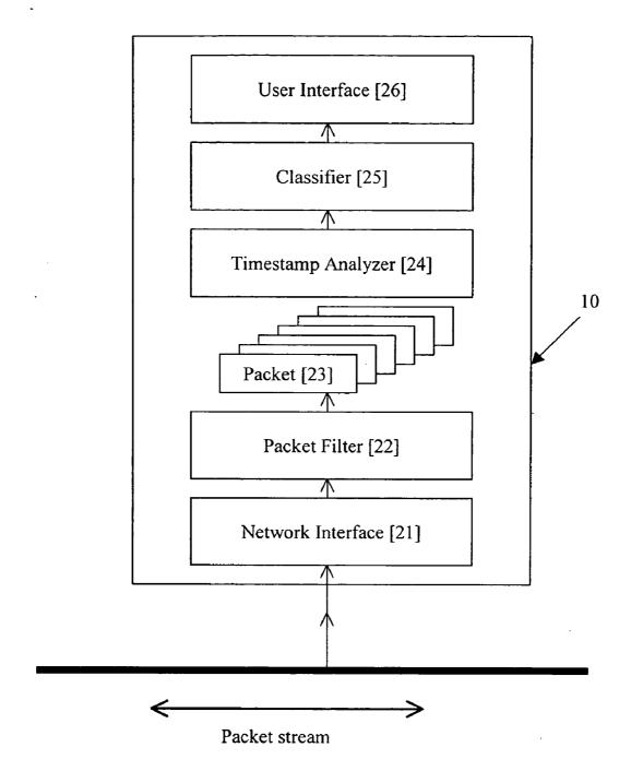
Figure 2. Descriptive diagram of System for Identifying and Locating Network Problems
