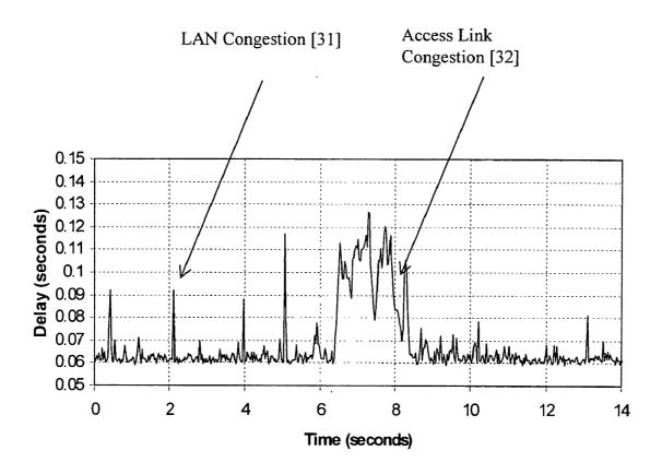
Figure 3. Example Network Delay Trace
