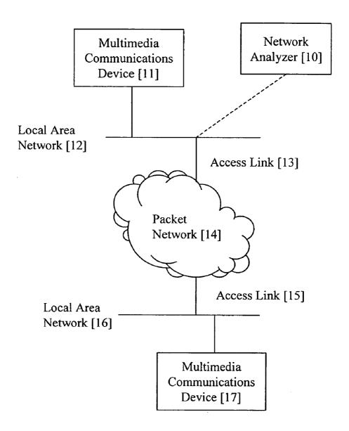
Figure 1. Example application of System for Identifying Network Problems
