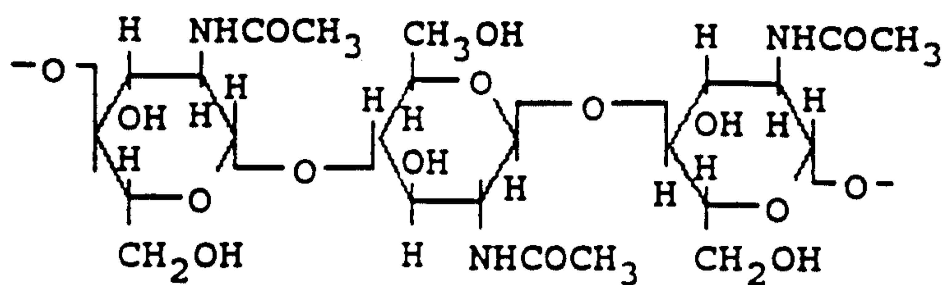
Chitosan has the formula (1->4)-2- amino-2-deoxy- $\beta$ -D-glucan, and has the following structure:
