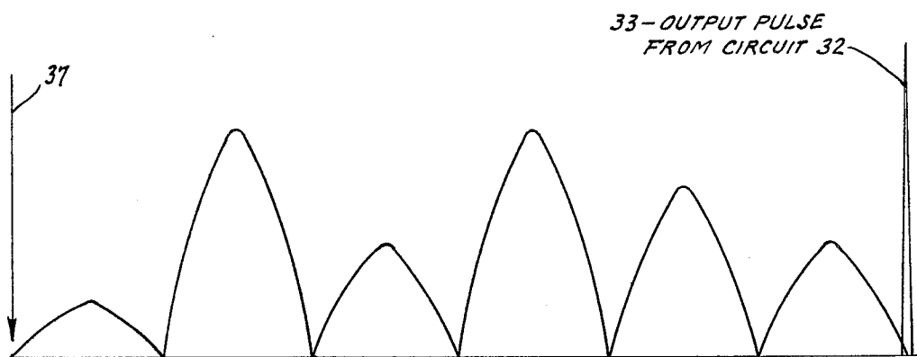
FIG 1C. RECEIVED SIGNAL ECHO FROM, TARGET AT ARBITRARY AZIMUTH (ALSO RESPONSE PATTERN OF CIRCUIT 32)
