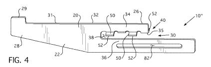
(57) Abstract: A support device is provided. The support device includes a support assembly with an elongated first body defining a cantilever mounting and a support surface. The first body cantilever mounting corresponds to the first flange. In this configuration, the first body may be coupled to the first flange and the support surface may be used to support a shelf.
