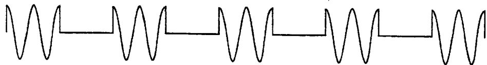
Fig 3: Alternative to pattern of Fig 2 with reduced field variation over active segments
