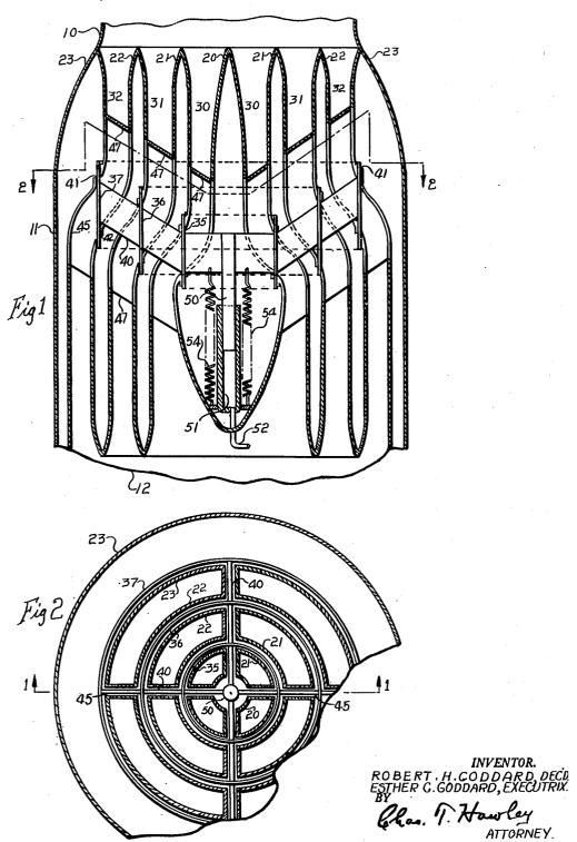
SLEEVE VALVE FOR RESONANCE COMBUSTION APPARATUS
