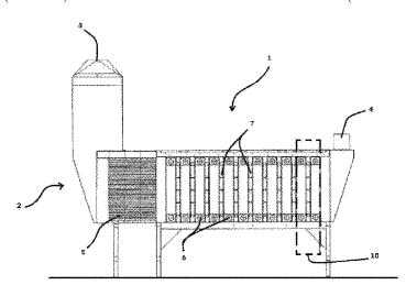
nanoparticle coating and the nanoparticle coating comprising titanium dioxide doped with a nitrogen doping agent. •a unit (5) for straightening the flow before the filtering unit (10).
