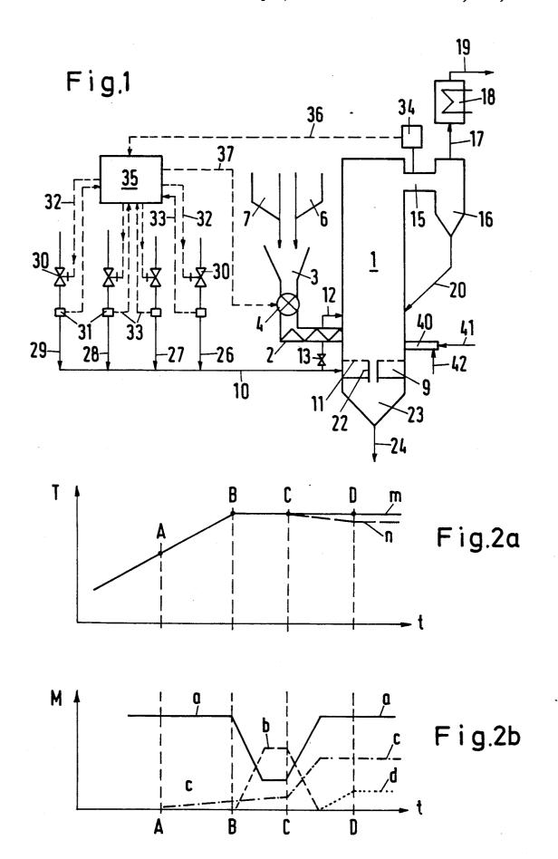
PROCESS OF CONTROLLING THE STARTING UP OF THE GASIFICATION OF SOLID FUELS IN A **FLUIDIZED STATE**
