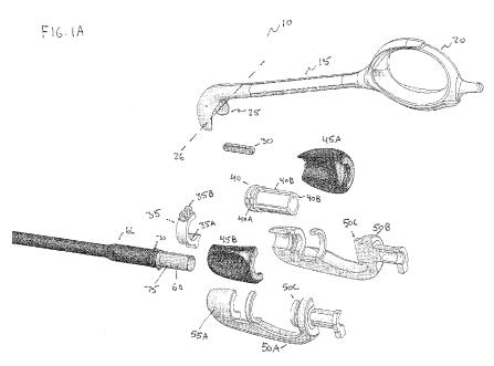
(57) Abstract: An energy-based surgical instrument is configured to permit selective cutting, coagulation, and fine dissection required in fine and delicate surgical procedures. The scissors grip instrument provides for tube-in-tube construction (60, 70) so the device is useful for both open and minimally invasive procedures. The assembly includes a clamping mechanism, including a clamp arm and/or housing which are specifically configured to create a desired level of tissue clamping forces.
