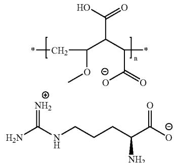
[0017] 1.0.3. Salt 1.0.2 wherein the methyl vinyl ether/maleic anhydride has a molecular weight (M.W.) of about 30,000 to about 1,000,000.
