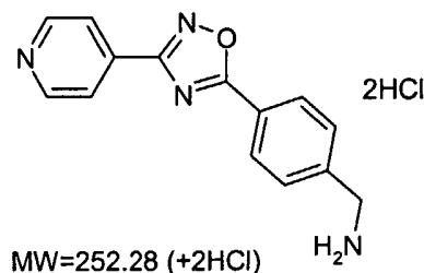
To a solution of 4-(Boc-aminomethyl)-benzoic acid (187 mg) in DMF (0.25 M) 10 were added DIEA (5 eq), TBTU (1 eq) and HOBr (0.2 eq). The solution was stirred at RT for 3 minutes, and then isonicotinamide oxime (102mg, 1 eq) was added. After 1 hour, the solvent was evaporated. The residue was triturated with 0.05 M NaOH (5 ml). The solid was filtered off, washed with water and dried under vacuum.
