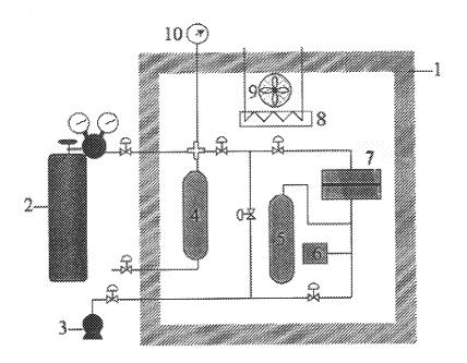
FIGURE 1. Schematic of gas permeation apparatus for flat membrane films
