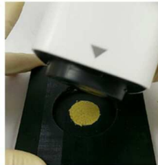
5. Fit the colorimeter into the tray
