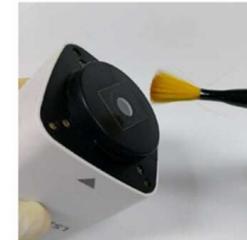
7. Gently clean the colorimeter with a soft brush
