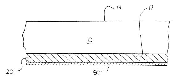
(57) Abstract: A substrate carrying a temporary protective cover and related methods of producing and processing substrates are described. In one embodiment, a substrate has a durable exterior surface bearing a temporary protective cover that protects the durable surface against contamination but that can readily removed from the durable surface by washing with a given washing fluid.
