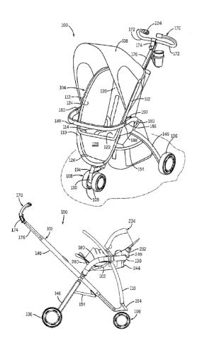
(57) Abstract: A is provide that is conf igured to transport interchangeable child seats. The stroller (100) includes a stroller frame (102) having a f irst set of connection locations (115) removably attach to a f irst child seat (104). The f rame also includes a removable child seat adapter (200) that can be connected to the stroller frame (102) such that the stroller f rame (102) presents a second set of connection locations that removably attach to a second child seat (234).
