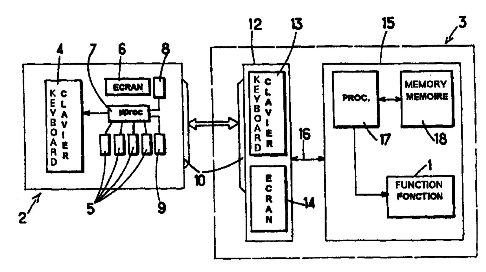
6,14... DISPLAY 7... MICROPROCESSOR 15... PROCESSOR Portable electronic device for safe communication system, and method for initializing its parameters.
