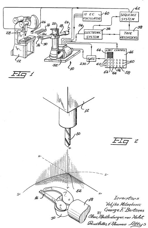
6 V. MILENKOVIC ET AL SELECTIVE CONDITION LIMITING RECORDING SYSTEM FOR A MOTOR CONTROLLED MACHINE TOOL
