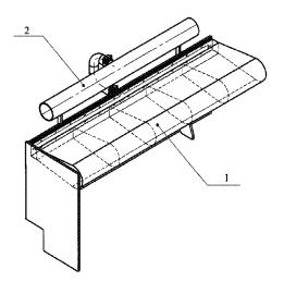
connect the airspace when deflated. In emergency mode the air supply to the air-inflated shutters is terminated, and the shutters get deflated and fully open the circular gap which ensures convection process throughout the whole area of containment building.
