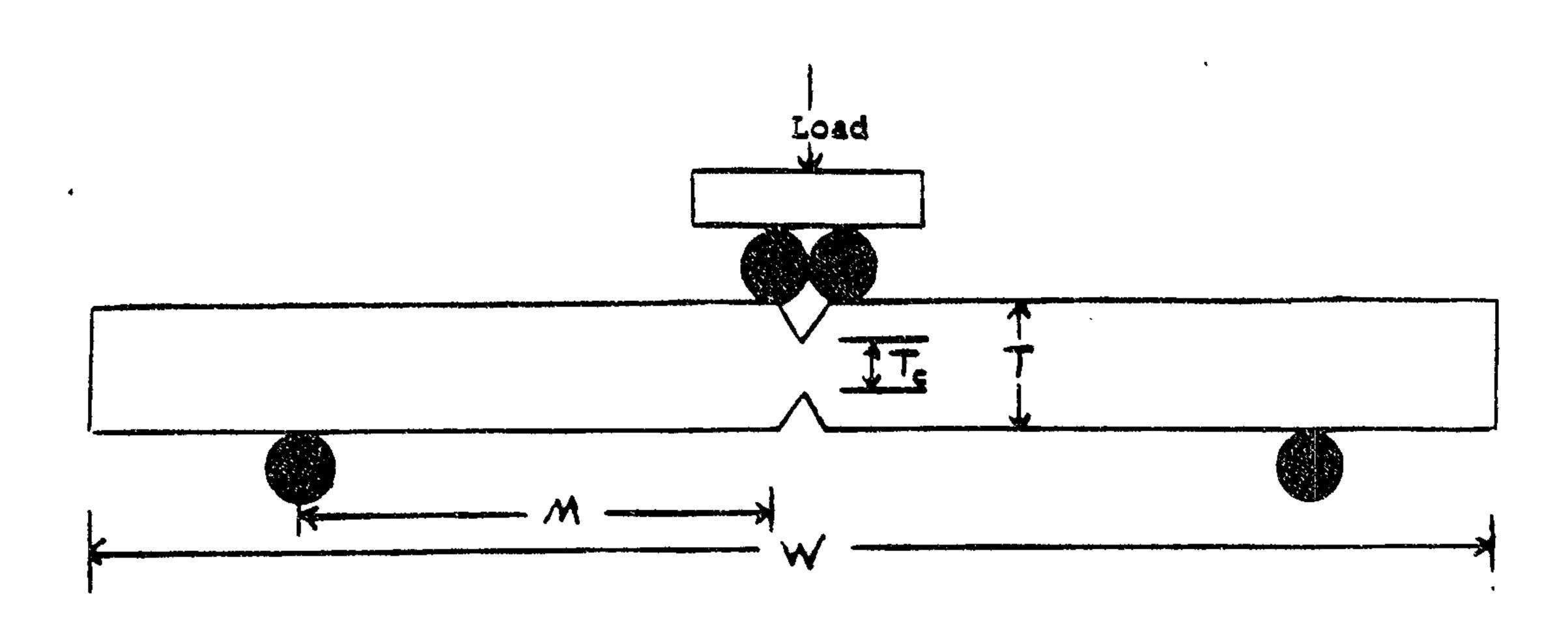
Typically there was stop/start propagation of the crack so that several peak loads, Pc, could be measured for each sample. The mode I fracture toughness,  $G_{lc}$ , was calculated according to:
