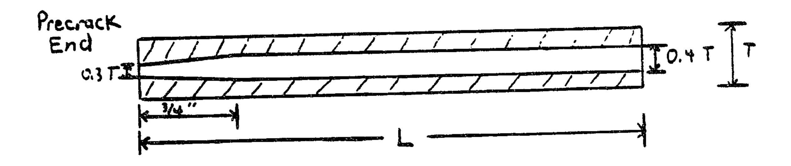
The sample was then precracked at the end bevelled to a depth of 35% of the thickness, by tapping a razor blade into the end. The beveled groove prevents the precrack from propagating the length of the sample before testing. The sample was then tested in double torsion as illustrated below.
