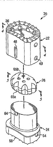
(57) Abstract: A vertebral implant device (20) for interposition between two vertebral endplates comprises an outer body (22) and an inner body (24). The outer body movably engages the inner body. A core (26) member positioned between the outer body and the inner body is at least partially compressed when a load is applied to the implant device.
