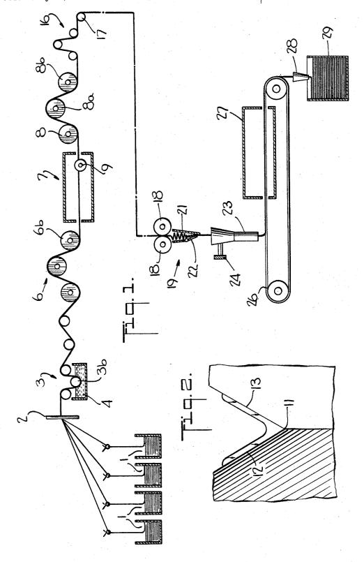
METHOD AND APPARATUS DEFLECTING AND DRAWING TOW
