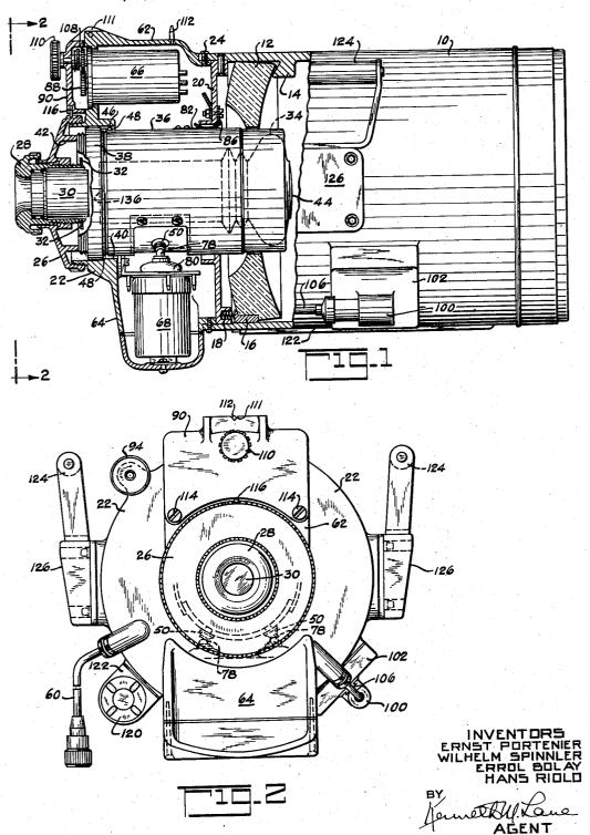
INFRARED IMAGE CONVERTER APPARATUS
