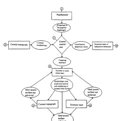
(57) Abstract: Apparatus for determining and ablating the corneal tissue volume for correcting visual ametropia, as optimized for each individual patient, whereby the apparatus comprises a central control unit (1) to which are operatively connected, either generally or partially, a corneal topograph (2), an infrared pupillometer (3), a scansion laser (4) and an excimer or solid-status laser (5).
