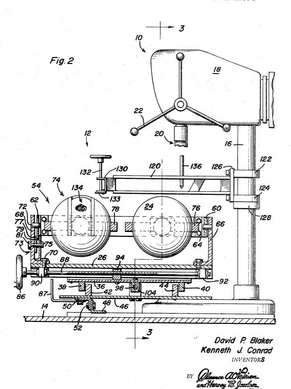
BOWLING BALL HOLE GAUGING DEVICE AND DRILLING APPARATUS
