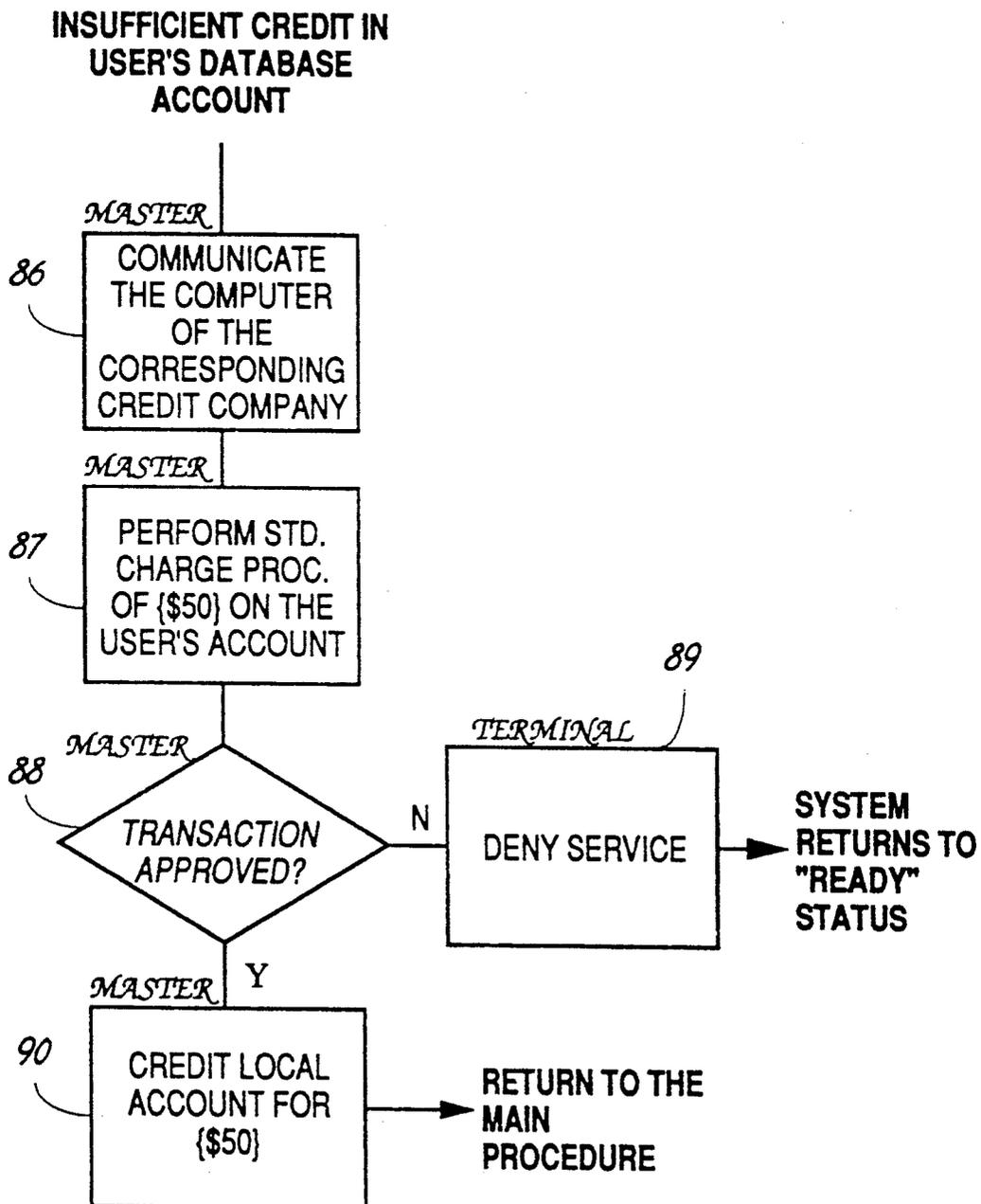
FIG. 7 — WRAP-UP Procedure
