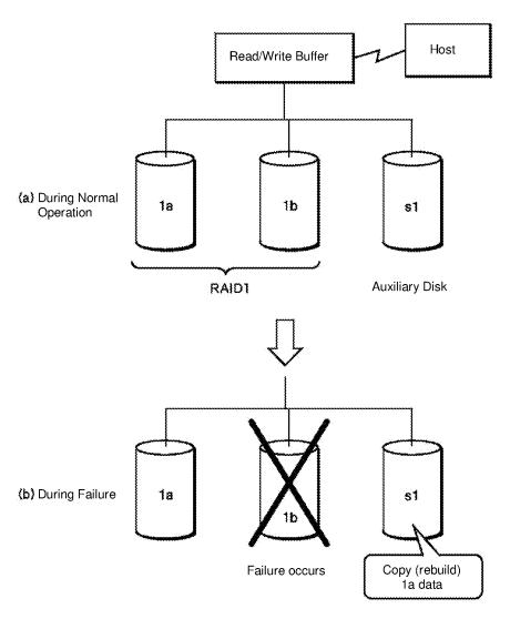
Notes • Auxiliary Disk: Used for redundancy of 1a instead of failed 1b
