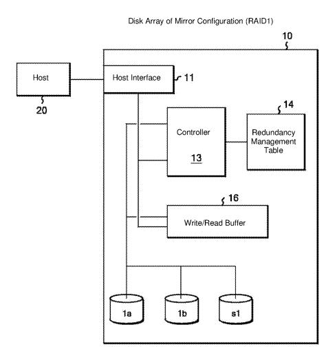
Notes • Mirror Configuration: Disk 1a and Disk 1b • Auxiliary Disk s1: Rebuilt when 1a or 1b fails
