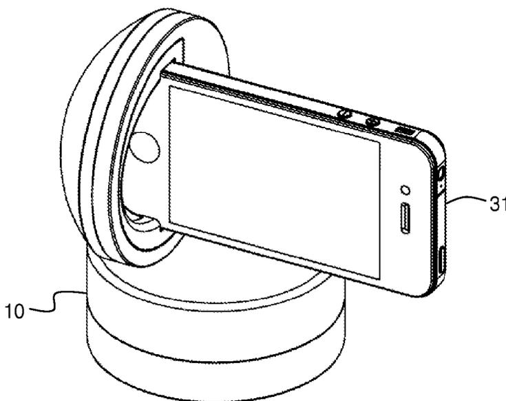
(57) **Abstract:** A multi-axis positioning device adapted to hold and position an electronic device such as a smart phone. A system using the positioning device and a smart phone adapted to utilize the smart phone to provide positioning commands to the positioning device. The system may provide positioning commands based upon pre-programmed instructions, or may position based upon analysis of the images being taken in real time.
