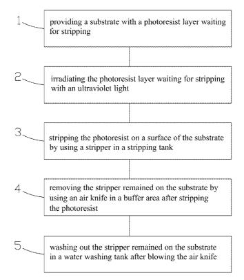
1 providing a substrate with a photoresist layer waiting for stripping 2. irradiating the photoresist layer waiting for stripping with an ultraviolet light З stripping the photoresist on a surface of the substrate by using a stripper in a stripping tank removing the stripper remained on the substrate by 4 using an air knife in a buffer area after stripping the photoresist 5 washing out the stripper remained on the substrate in a water washing tank after blowing the air knife
