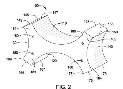
(57) Abstract: Apparatus and methods for supporting one or more elongated members are provided. A support member for supporting one or more elongated members can include a body; at least four support arms extending from the body, and at least one curved surface disposed between the support arms. Each curved surface can be concave relative to a centerline of the body. At
