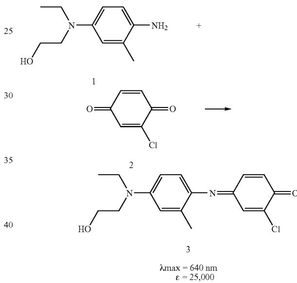
The components in the coating layer react under second UV exposure to erase a formed image by reversing the reaction of forming the extended conjugation compound (3)
