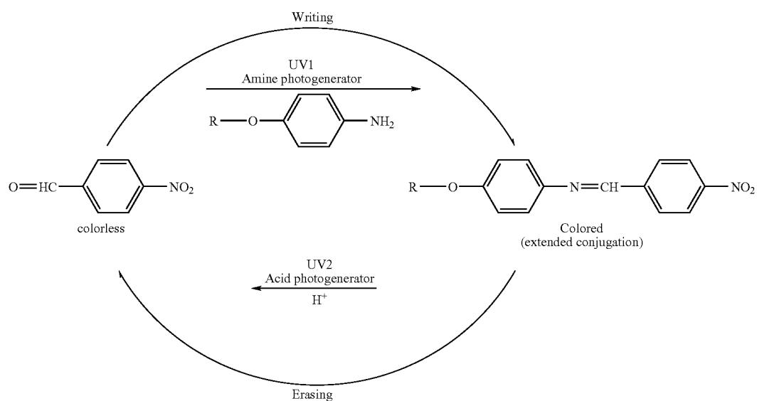
In general, any coupling agent that produces a significant enough color change upon reaction with the generated base, and which reaction and color change is reversible upon reaction with the generated acid, is suitable. Exemplary coupling agents include aldehydes, ketones, and mixtures thereof. For example, suitable aldehydes that can be used include adoxal, anisic aldehyde, cymal, ethyl vanillin, florhydral, helional,
